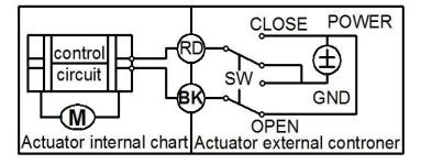
• RD connect with positive, the BK connect with negative, the valve closed, the actuator automatically power off after in place, the valve remains fully closed position .
